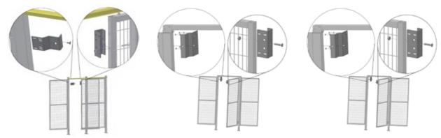
The mounting plates for safety switches have a universal mounting system that is suitable for most switch manufacturers' products. They are easily installed on the relevant door solution and extended
