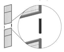
If the installation in your **Arion Pro-Tect** machine safety system requires higher walls than our **ProSafe** standard panels permit, our panel extension kits allow the height to be increased. The extension kit makes it possible to install two ProSafe panels on top of each other. We do not however recommend increasing the standard heights by more than 1500mm. (If your installation requires greater height, we recommend that you contact us so that we can provide specially made panels.)
