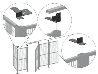
Our consoles for cable ducts are very simple to install on top of the uprights in your **Arion Pro-Tect** machine safety system and make it possible to secure cable ducts to simplify installation and keep cables in order.
