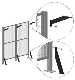
If your **Arion Pro-Tect** machine safety system layout requires extra support for the uprights (for example long freestanding walls or large, heavy doors) our support brackets give the opportunity for stabilising uprights either at the floor or roof. We recommend using the support brackets when a freestanding wall exceeds 5 metres in length.
