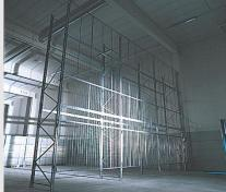
The Anti-Collapse System represents a simple but yet cost effective method of avoiding many accidents in the storage and handling of pallets in and on racking systems. The framed mesh system is mounted on brackets, which are designed to fit most types of racking systems. The brackets range from 100mm to 250mm in length, other sizes can be manufactured to your requirements. The mesh panels are available in mild steel powder coated but RAL colours can be supplied to order.
