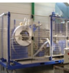
Installation with single mesh panel and fittings of painted metal
