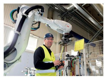
500 kg and torque equivalent to 5,000 Nm. The modularity is extensive, and the peripherals can entail everything from materials handling to bonding and spot welding. MQC is an abbreviation of Manual Quick Changer, used to facilitate manual tool changing.
