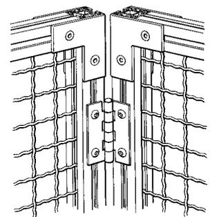
**Note!** The JSM 35-K must only be used for making fence angles.
