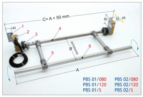
Multi-function item, particularly strong and with various adjustments, suitable for use on different types of machines - Based on the purpose for which it is installed, it allows to operate the "Stop - Start" system, for the simple stopping and-or starting routine, or the "emergency" system for unexpected dangerous situation - Available with single microswitch, code PBS 01/... (assembled on the Left box and, if necessary, shifted on the Right) or with double microswitch, code PBS 02/....
