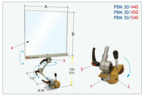
Magnetic fastening item for universal use, suitable to be used on metal work surfaces and machinery bases - Its numerous articulations allow a shield positioning in any direction: vertically - horizontally "flag type" - with its upper end in contact with the base.
