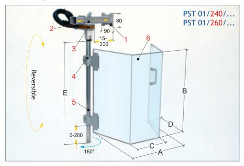
Protects the operator from direct contact with alternate moving parts of the vertical slide and from the projection of shavings.
