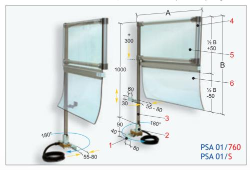
Protects the operator from direct contact with alternative moving parts of the cut group accessible sideways as well as from the projection of metallic parts that could be generated. Posteriorly attachable on the two sides of the base - The shields are subdivided into two sections, the lower one is made of flexible Pvc, to be potentially shaped for the passage of rods in working. Complete with safety microswitch.
