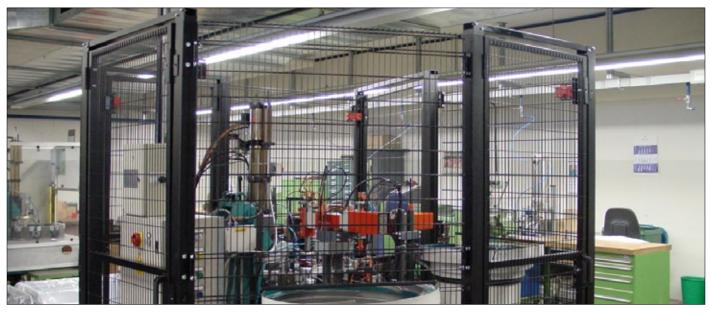
**Arion SmartSafe**<sup>™</sup> A simple and strong system with mesh panels which are frameless but with folded edges on all 4 sides to increase its overall strength. Otherwise it has the same construction as RAPIDSAFE safety fencing systems.
